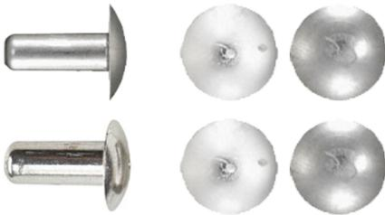
**FULL BRAZIER HEAD SOLID ALUMINUM RIVETS** Full brazier head gives a larger bearing surface under the head resulting in a greater resistance to pull through; Available in hard or soft aluminum.
